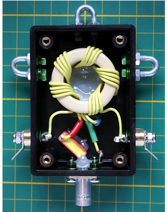
This balun is boxed into ABS enclosure. *Do not use metal enclosure for high-impedance baluns!* Output connectors are 6,3mm Abiko terminals and the coaxial connector is a standard BNC female with flange. The enclosure may be potted with beeswax or epoxy.
